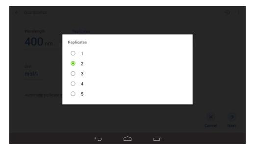
If 2 or more replicates are selected, Automatic replicate measurement becomes active. Automatic replicates will read the same sample for the selected number of replicates. If individual sample replicates are being used, do not select the automatic replicates option.
