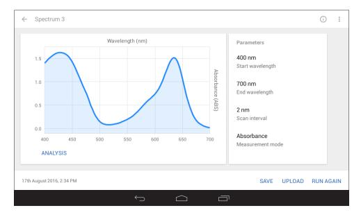
Once the spectrum scan is completed it is possible to analyse the spectrum scan. Post measurement tools include peaks and valleys and area under the curve. To analyse the data touch **ANALYSIS**.
