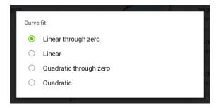
The curve statistics are also displayed for the curve fit chosen. For example if the curve fit is y = mx+c the curve statistics displayed will be the gradient of the line (m), constant (c) and correlation coefficient (r<sup>2</sup>).
