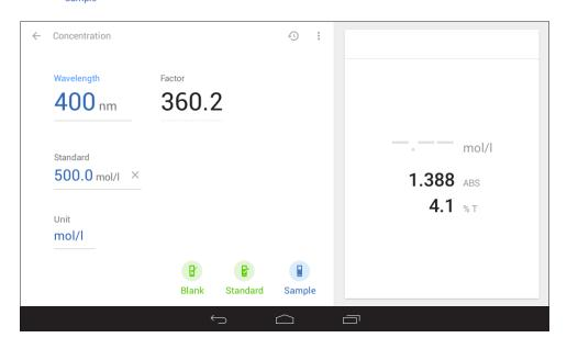
The spectrophotometer will calculate the factor so that this value can be used for future measurements.
