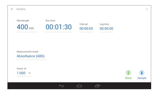
If a lag time has been set the instrument will count down the lag time before the kinetics run starts. If no lag time has been set the kinetics run starts straight away and a live kinetics run is shown on the screen.
