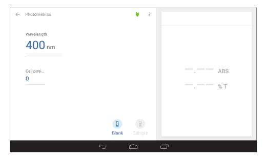
Set up the required measurement parameters. Insert the cuvette containing the blank solution into turret position 0 followed by the cuvettes containing the samples into turret positions 1 to 7 and close the instrument lid.
